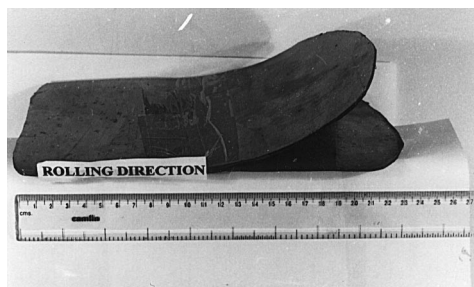
Fig. 2. Failure of AR material by alligatoring after about 40% reduction at room temperature rolling.
